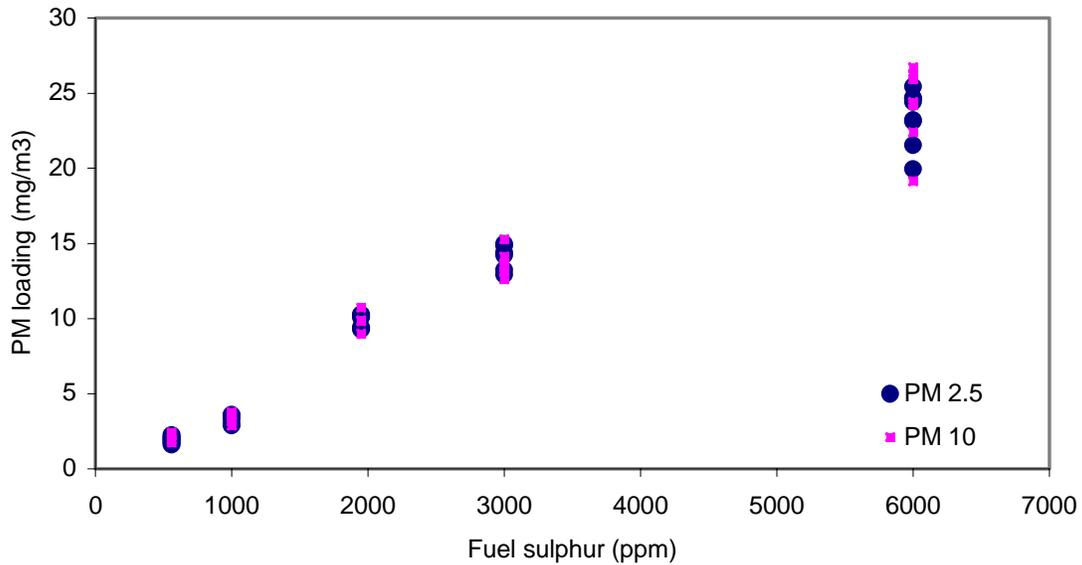
**Figure 2-2 Effect of fuel sulfur on PM<sub>2.5</sub> and PM<sub>10</sub> emissions**
