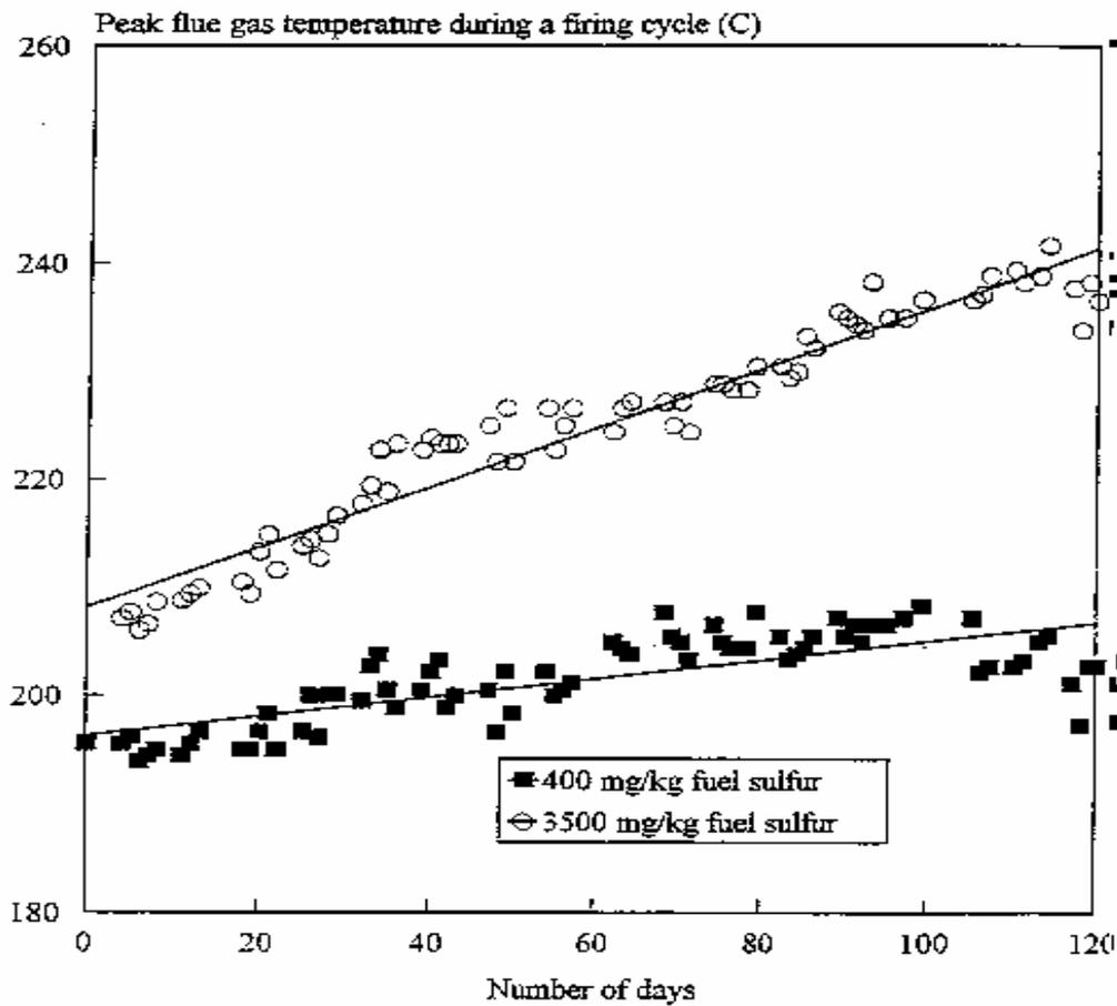
Figure 6. Trends in peak flue gas temperature during full size boiler tests.
