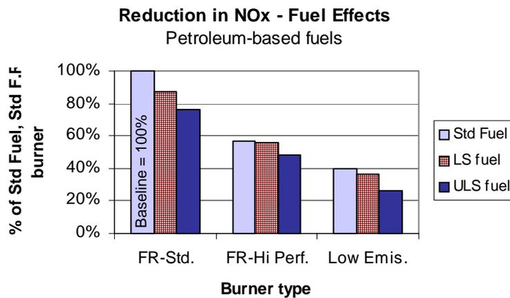
Figure 2-3 Fuel sulfur effects on NO<sub>x</sub> formation
