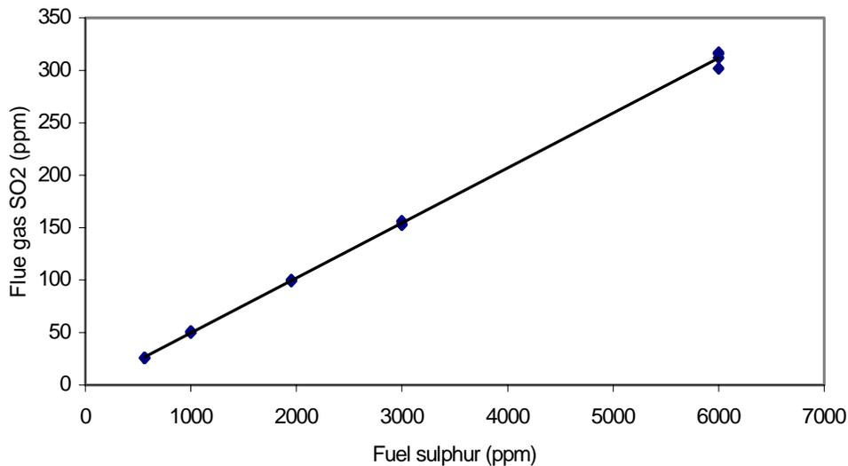
**Figure 2-1 Effect of fuel sulfur on flue gas SO<sub>2</sub> emissions**
