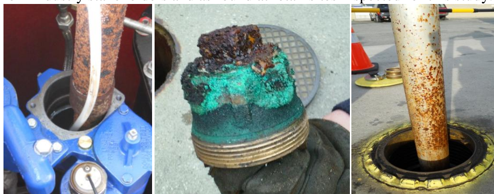
Figure 1. Corroded ULSD equipment: Corroded carbon steel submersible turbine pump (STP) shaft removed from pump housing, CA-1 (left), brass ball float extractor cage plug, NY-2 (middle), aluminum drop tube, NC-1 (right).
