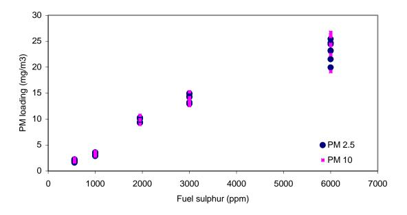
Figure 2-2 Effect of fuel sulfur on  $PM_{2.5}$  and  $PM_{10}$  emissions
