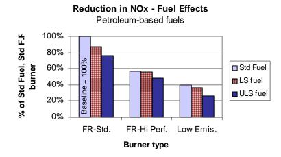
Figure 2-3 Fuel sulfur effects on NO<sub>X</sub> formation
