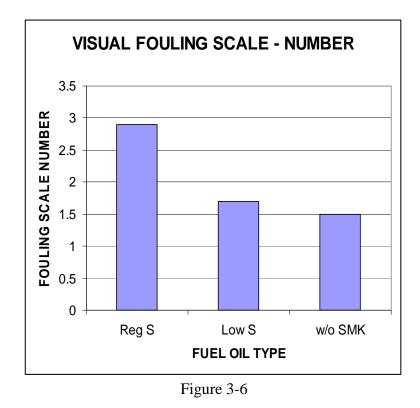
A similar difference in fouling factors was obtained for approximately 100 normal and low sulfur homes that did not have their deposition rates measured (Figure 3-6). The average Visual Fouling Scales for the Normal sulfur homes in this group was 2.6, and for the low sulfur homes was 1.7. The visual fouling scale appears to accurately predict the measured deposition rates, and gives similar difference when comparing the normal and low sulfur fuels.
