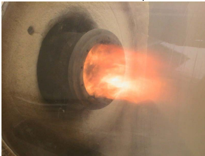
Figure 14) FFA fuel (processed trap grease) firing in a residential oil burner in tests at Brookhaven National Lab. Fuel temperature is 230 F.
